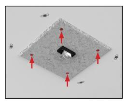
11. Secure the board to the drywall bracket using the provided screws.
