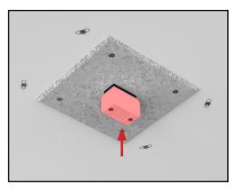
12. Take the reflector guard and carefully reinstall it to the fixture. The fixture must remain off for the remainder of the installation.
