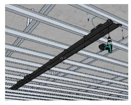
5. Lift the profile composition and install the composition to the framing.
